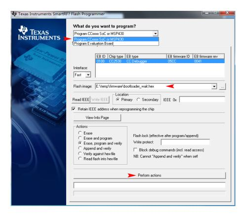
• When finished, there will be a message "Erase, program and verify OK" appears on the bottom of the window, and the LED1 of the baseboard will keep blinking indicating that program downloading is successful.
