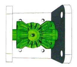
This set of bevel gears is designed for situations where a drive shaft needs to change direction or branch out at 90 degrees. The medium duty bevel gears will press fit onto a 2mm (5/64th) diameter shaft but can be drilled out to suit shafts up to 4mm (5/32nd).
