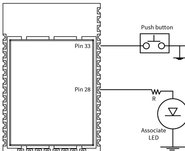
A pushbutton and an LED can be connected to XBee/XBee-PRO S2C ZigBee RF Module pins 33 and 28 (SMT), or pins 20 and 15 (TH) respectively to support the commissioning pushbutton and associate LED functionalities.
