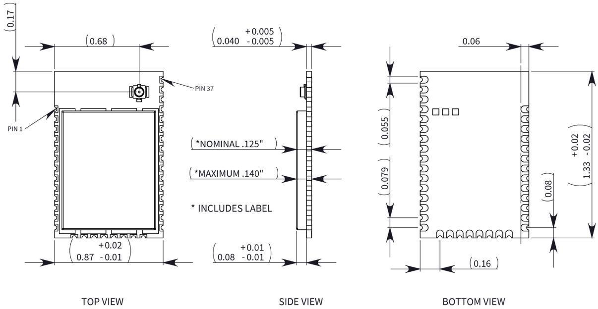
The drawings below show the XBee-PRO through-hole model.
